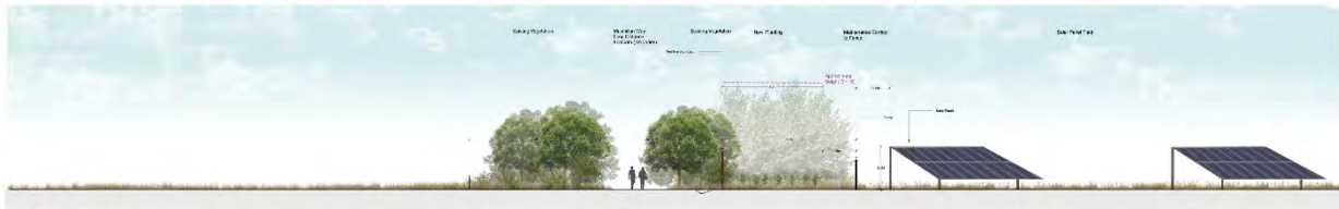
Section 2: E02 - Woodland Section shows new planting to supplement existing and screen the Solar PV development from the Woodland Way Long Distance Footpath. New planting heights indicated at year 1 and year 15.
