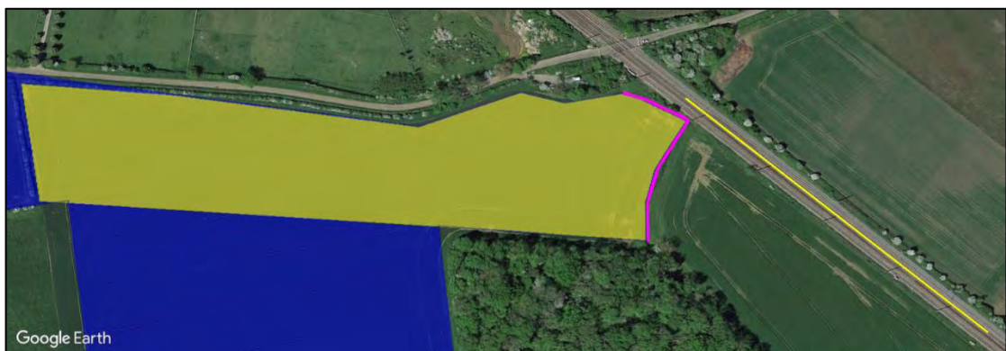
Figure 30 Reflecting panel area and potential screening location for train driver receptors 47 to 50 (fixed)
