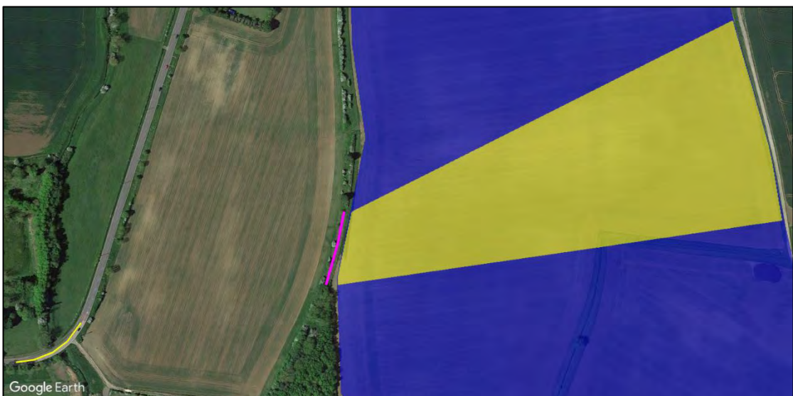
Figure 26 Reflecting panel area and potential screening location for road receptor 64 (fixed)
