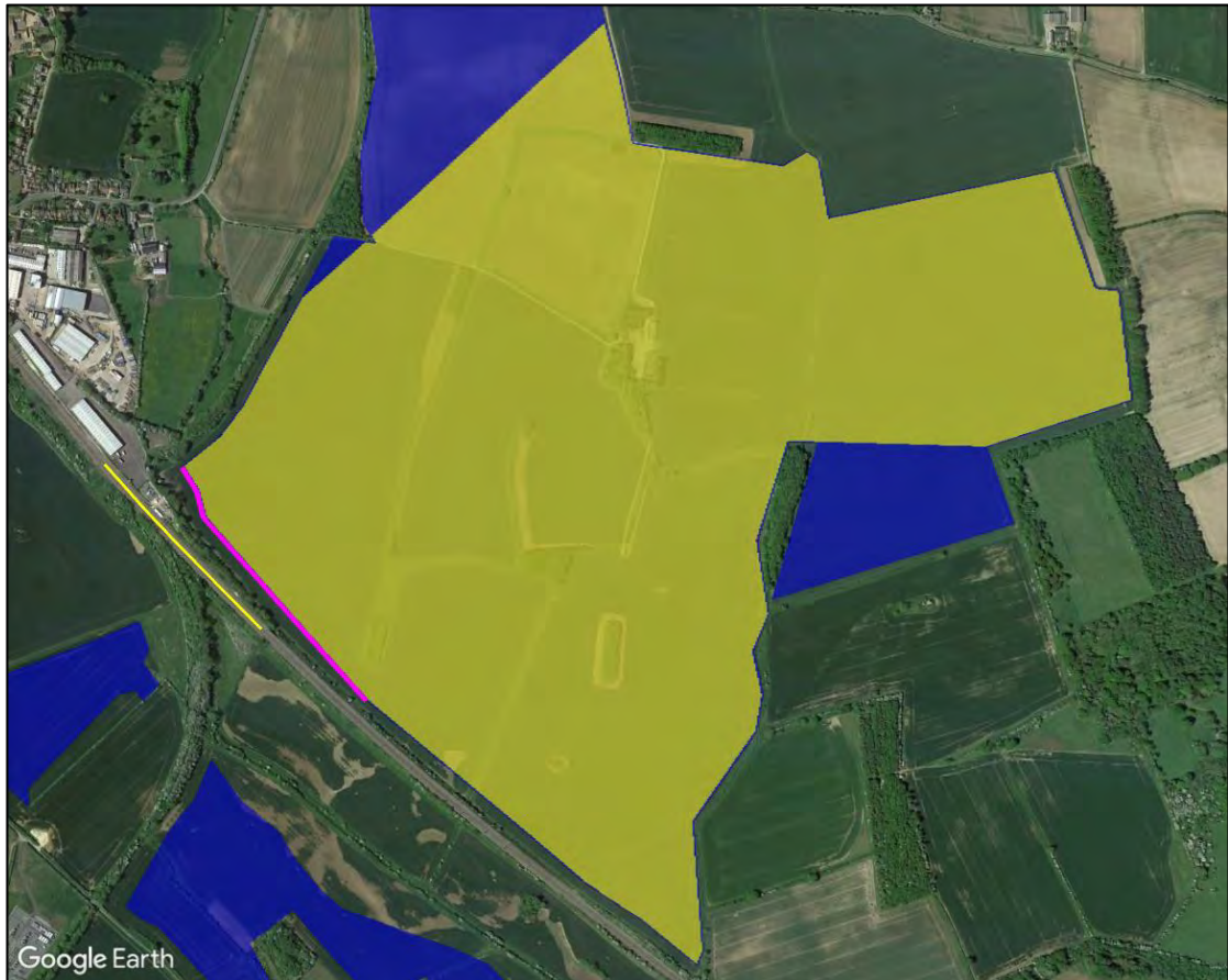
Figure 31 Reflecting panel area and potential screening location for train driver receptors 24 to 28 (tracker)
